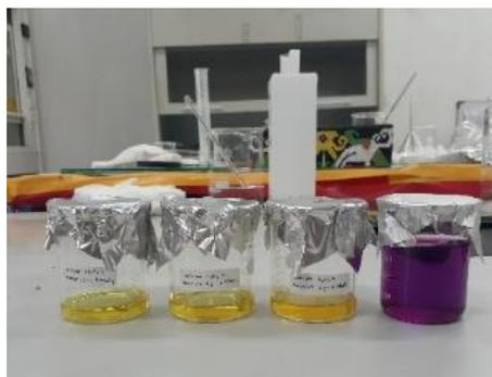
**Fig 1.** Color Solution of Ammonium Molybdate and Potassium Permanganate
