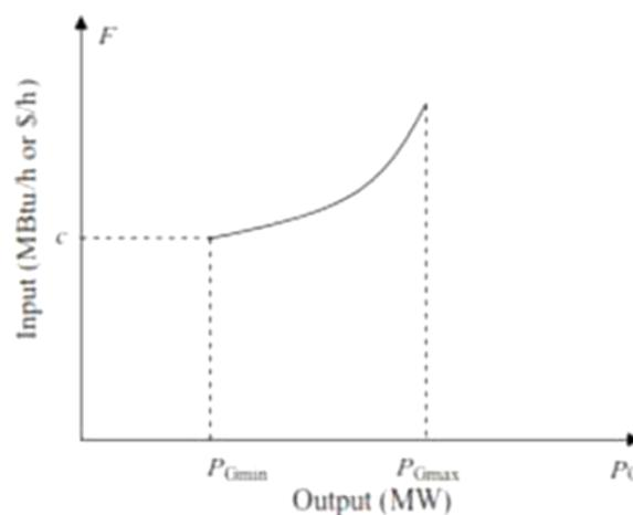
**Figure 1.** Input-output characteristics of the generating unit
