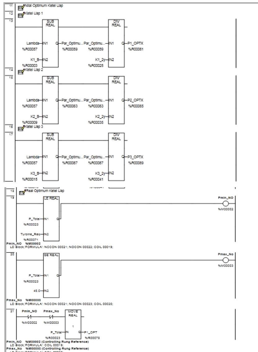
**Figure 7.** The ladder diagram section for the optimum value of the boiler output. The HMI programming used for this research is a control system of a process for controlling the boiler output flow. HMI programming on this boiler system is shown in Figure 8.
