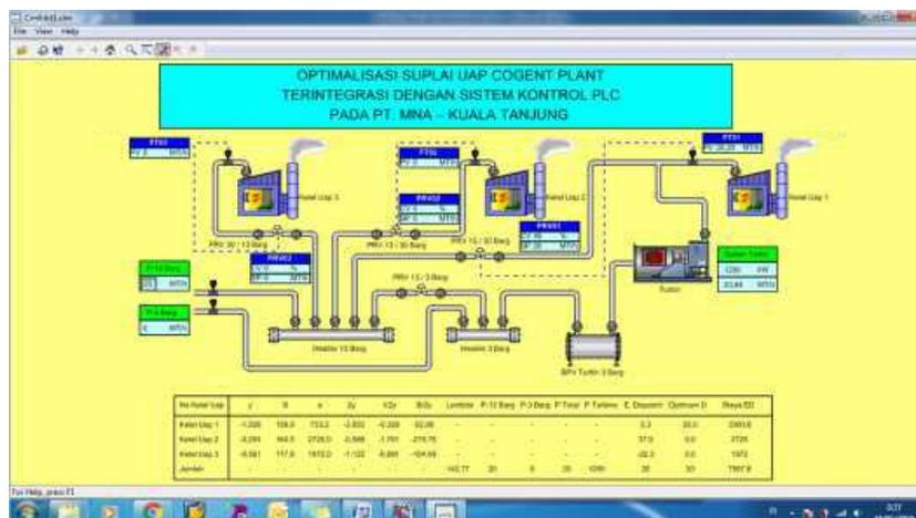
**Figure 8.** HMI of the steam supply system
